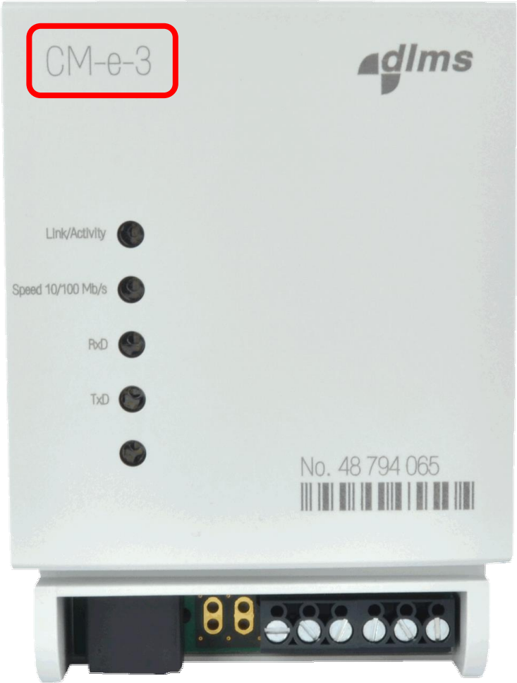
Figure 21: CM-e-3 module type designation
