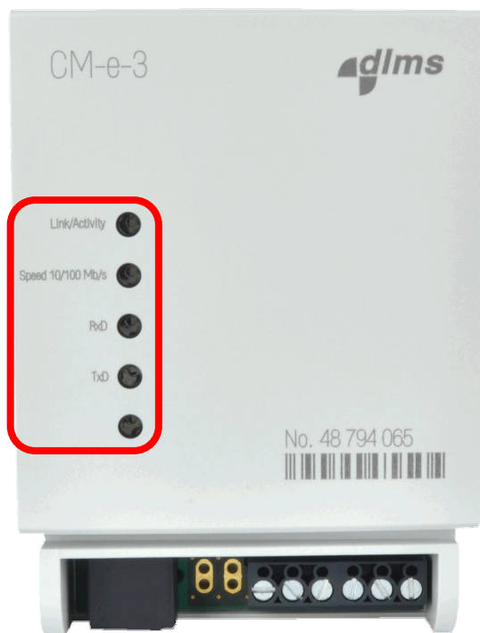
Figure 19: LEDs position on the front plate
