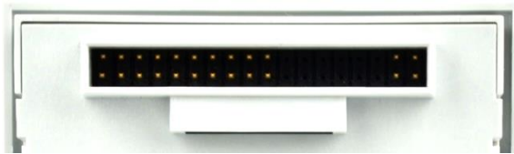
Figure 2: 24 pin connector on the back side of the module
