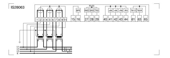
Note: Auxiliary terminals 27, 28 and 29 are implemented in RJ11 connector (see chapter 2.7).
