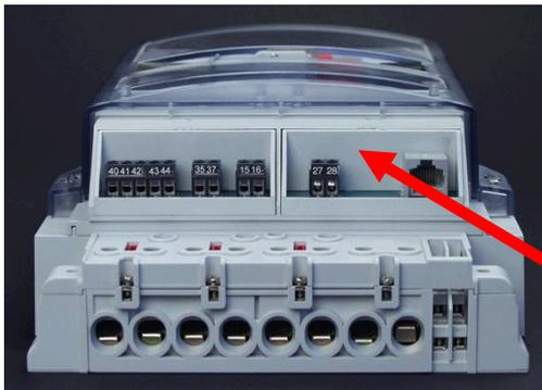
The MKMB-3-e-3 module fits into the right slot of the meter, as for all the other communication modules
