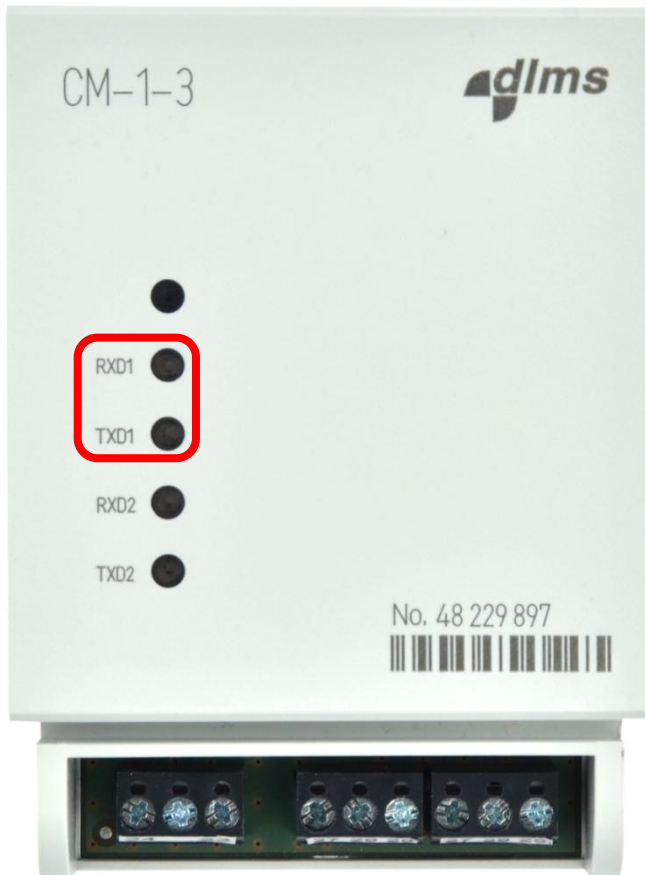
Figure 3: Primary communication channel LEDs position on the front plate
