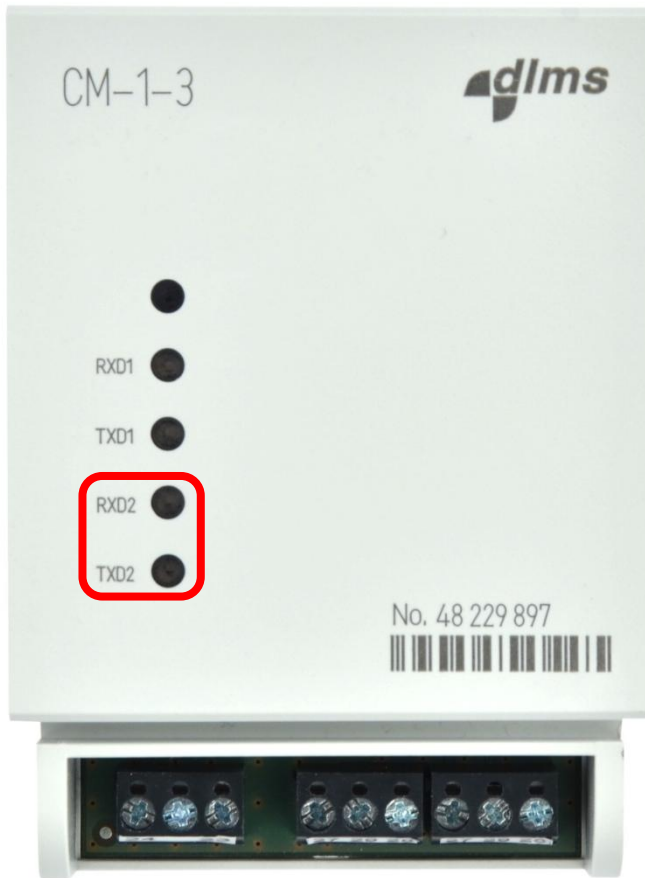
Figure 4: Secondary communication channel LEDs position on the front plate
